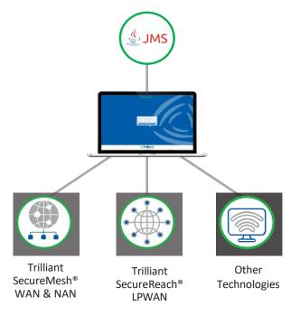
Trilliant's next-generation network technologies encompass Wide Area Networks (WAN), Neighborhood Area Networks (NAN), and Low Power Wide Area Networks (LPWAN). These technologies communicate with the HES through the Smart Energy Access Layer (SEAL API). The Java Message Service<sup>®</sup> (JMS) API manages messages, stores events, data, etc. for end users to evaluate.
